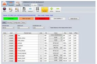
This plugin ads support for our own DS-IMU (Inertial Measurement Unit) next generation navigation instruments. If features up to 500 Hz output data rate and complies to IP67 & MIL-STD-810G environmental protection. It is synchronised with all other DEWESoft devices and input sources.
