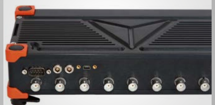
8 BNC connectors on rear side for analogue output.
