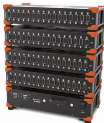
Typ. configuration : single or multiple slices(s) combined together with powerful SBOX and new 12" high brightness Display
