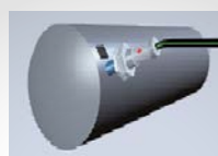
With an optical tach probe (1 pulse per rev) on a reflective sticker angle and RPM can be calculated.
